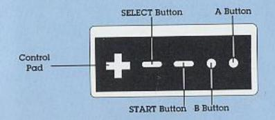
The control pad: This bad boy will move the boxer around the screen (press it either left or right to advance or retreat, up or down and diagonally to strike.) The control pad will also take you from "option" to "option" on the menu screen and "Select Hits" modes. (The control pad can also be used to cycle through all selections in any given "option."
